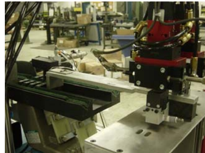
Linear Discharge w/ Active Orientation Tooling
