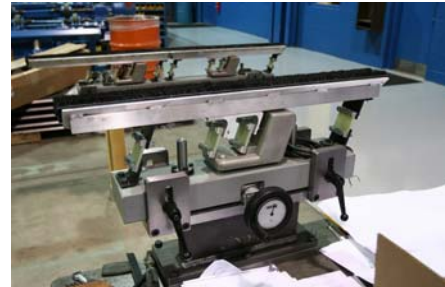
V-Track Discharge w/ Precision Adjustment
