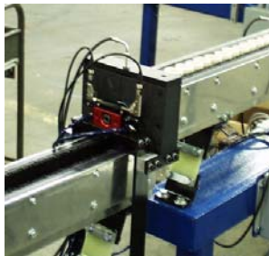
Accumulation Discharge w/ Singulation Escapement
