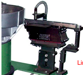
Gravity Track w/ Singulation Escapement
