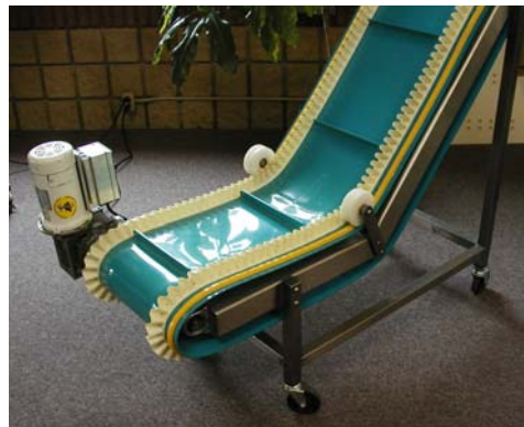
Direct Drive= Versatile Motor Location
