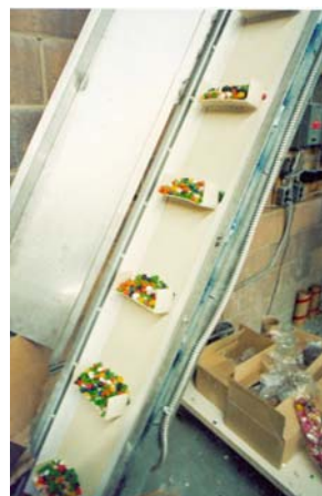
Steep Angle Incline w/ Flights for Candy Handling
