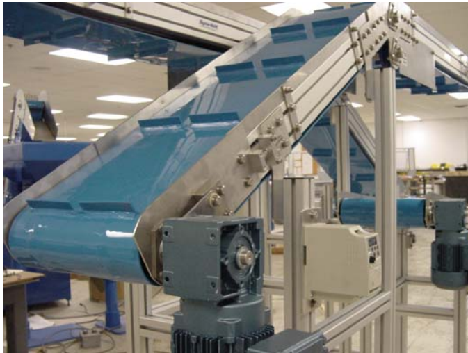
Direct Drive= Versatile Motor Location
