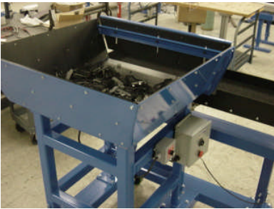
Pans include manual or automated Product Flow Gates
