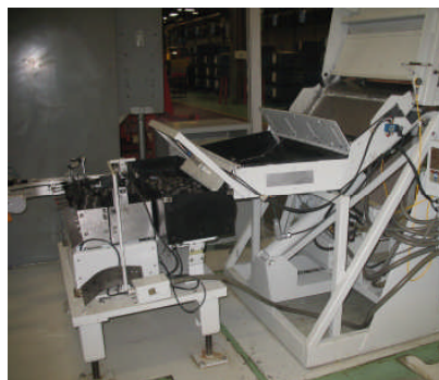
Automated Dunnage Dumper Supplying parts to intermediate pan w/ flow control gates.
