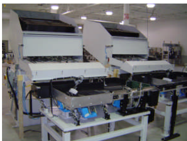
Automated Dunnage Dumper Supplying parts to intermediate pan w/ flow control gates.
