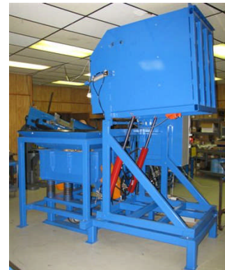
4,000 lbs Metal Castings in Steel Dunnage Smart-Dumper Automated Flow Control Gate Integrated with HD Pan Feeder
