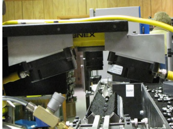
Vision –Pattern Recognition & Selection Carbide Bit Orientation to Grind Process
