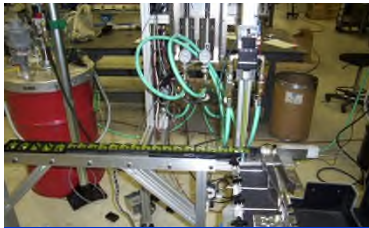
Electronic Part -Oriented and meter fed to OEM Substrate Dispenser
