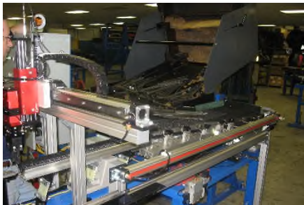
Part feed from integrated bulk supply, fed & oriented to defined end leading and the automatically to Lathe
