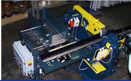
Magazine Tube Feeder Supplying Parts to rifled V-Tack Feeding Chamfer & Trim Machine
