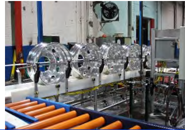
Aluminum Truck Wheel Oriented and metered to Conductive Test Cell
