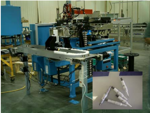
Assembly Pallet Loading System Spark Plug Bodies- 60ppm
