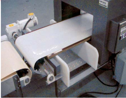
Metal Detector & Reject Station.
