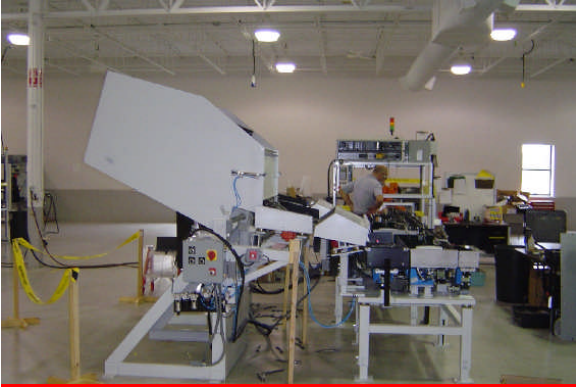
Reduction pan feeder integrated to dumper
