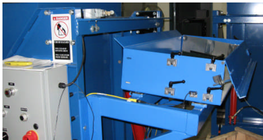
Intermediate Reduction Pan w/ Adjustable Side Guides and Flow Gate Absorbs impact load-meter parts/materials.
