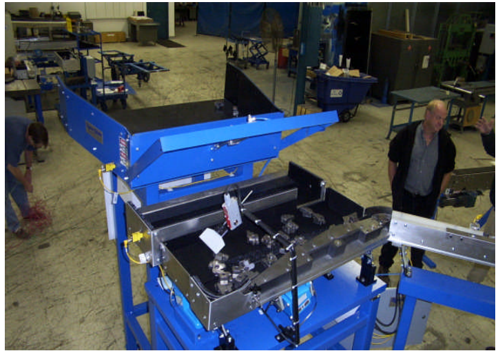
Pan integrated to existing high level dumper
