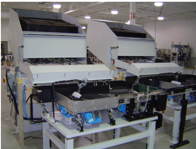
Multiple "smart dumpers" w/ flow control pans in operation. Integrated to robot assembly cell.
