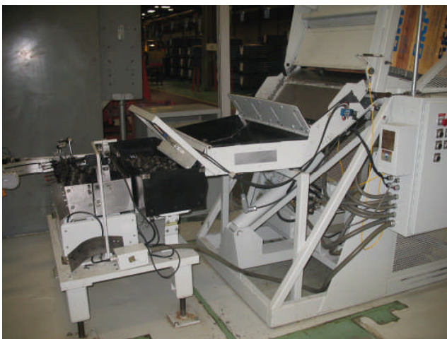
Receiver Pan Feeder w/ active pan for receiving parts dumped from portable bulk containers. Pan absorbs impact load and is integrated to dumper with manual or automatic flow control gates to effectively meter parts to "on demand" upstream systems.
