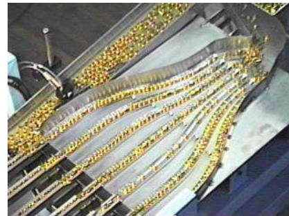
"Star Pan - Tooled Pan for lateral distribution of parts, packages or materials"
