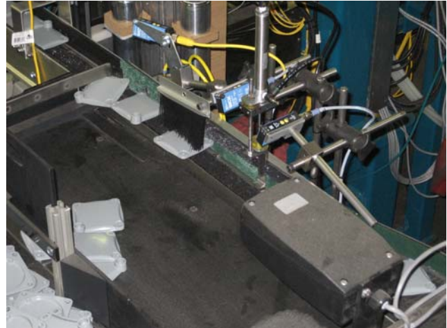
Sensor array to actively seek part features and actively sort off parts with incorrect orientation.
