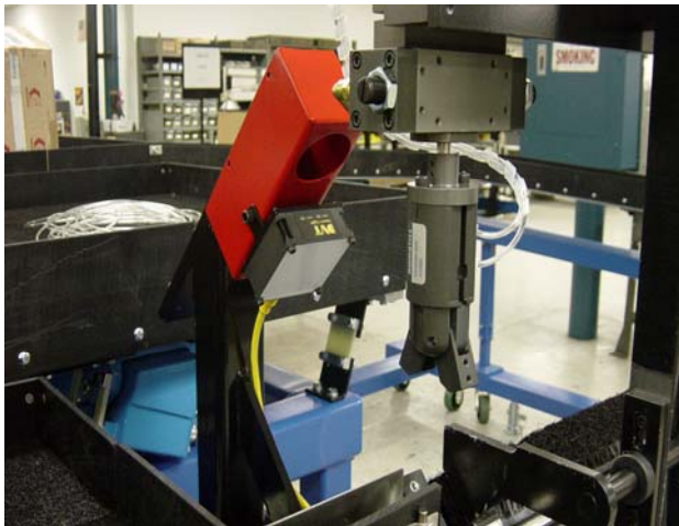
Vision Guided Orientation to orient parts that lack either features or geometry which will allow the use of passive tooling.
