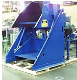
Multiple Products-Automated Dunnage Dumper Supplying parts to intermediate pan w/ flow gates. Parts supplied to Robotic Assembly Cell on demand
