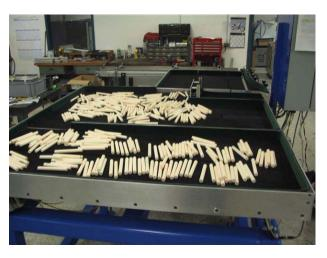
System is designed to accumulate up to 600 parts. To accommodate this large number of parts without damage required segmenting accumulation table into zones. Each zone is segmented using pneumatic gates. Gating the zones had the added benefit of allowing positive part separation to be maintained between grind cycles.
